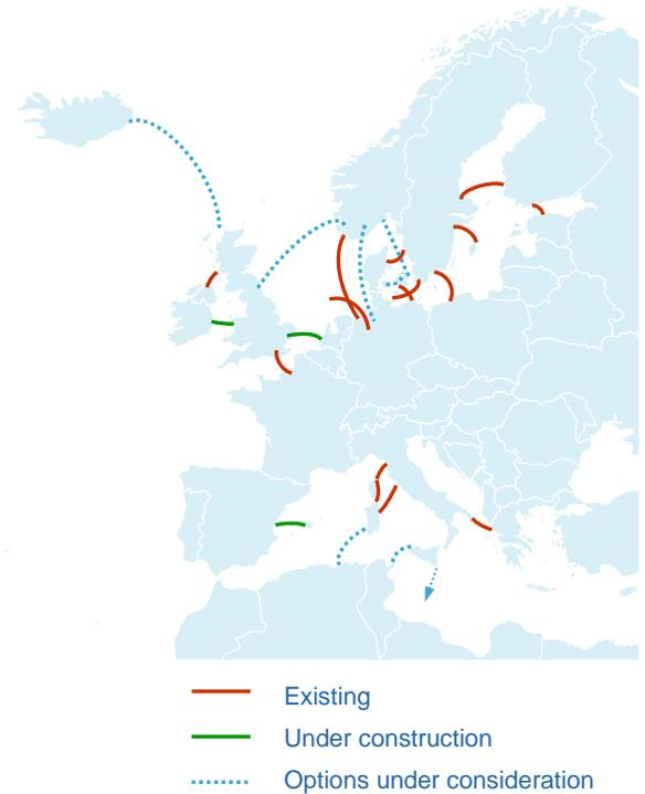
**Figure 13: Trans-boundary HVDC interconnections in west Europe**
